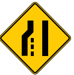
Pavement Width Transition Left S3030W42L(H)A S3636W42L(H)A
