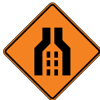
Double Pavement Transition S3636W42D(D)AC S4848W42D(D)AC
