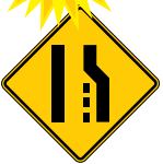
Pavement Width Transition Right S3030W42R(H)A S3636W42R(H)A
